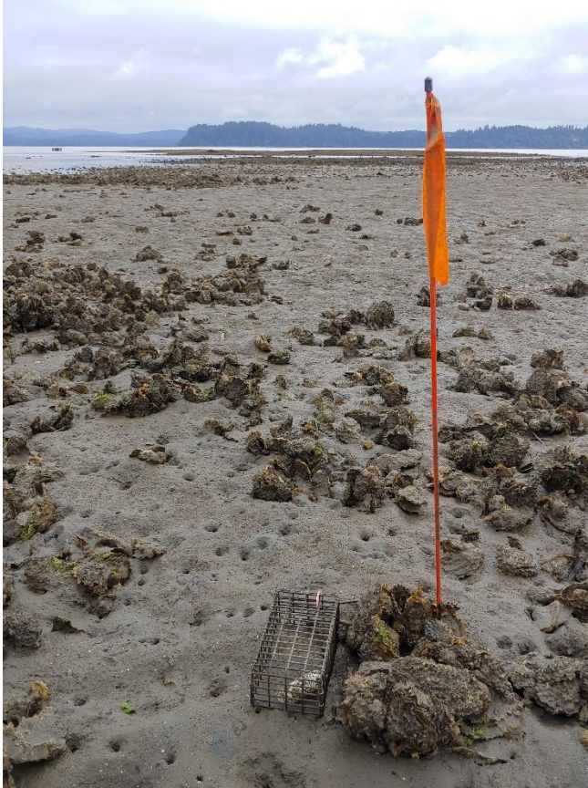
Figure 8. Vp sample site in Nahcotta, WA with orange flag marker and USB data logger enclosed in a small cage. Photo credit: the author.
